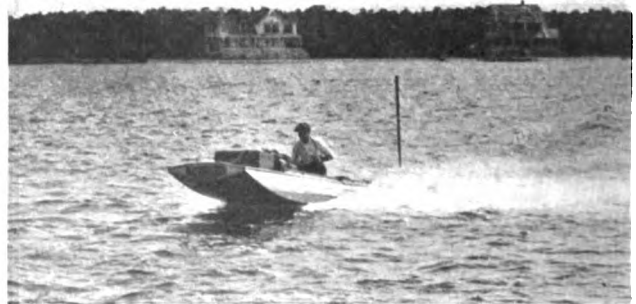
Snapshot, a 16-Ft. by 3½-Ft. Hydroplane Powered with a 12-H.P. Kermath Motor. Her Speed is 21 M.P.H. and She is Owned by Her Builder, Mr. R. K. Pearce of Islands Heights, N. J.
